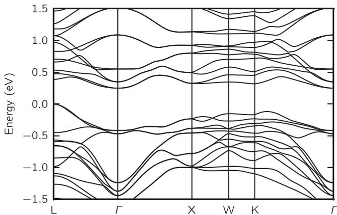
FIG. 2. First-principles fully relativistic computed band structure of  $\text{Zn}_2\text{Os}_2\text{O}_7$  with partial Te substitution ( $\text{Zn}_2\text{Os}_2\text{O}_{6.5}\text{Te}_{0.5}$ ).
