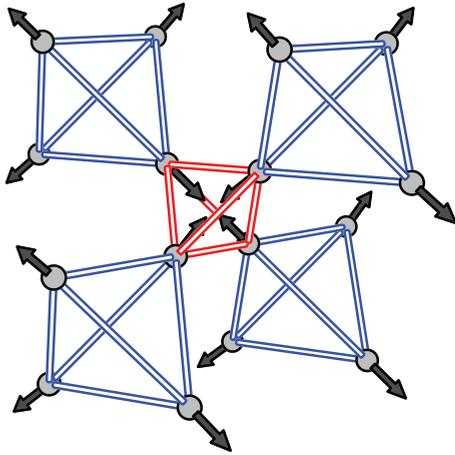
FIG. 1. (Color online) Sketch of one out of 30 canonical structures in which isotropic ME coupling  $\alpha^{\text{iso}}$  is allowed by symmetry. Atoms (gray spheres) are displaced in the direction of their magnetic moments (arrows). These displacements change the network of corner sharing tetrahedra by shrinking half of the tetrahedra (red) and enlarging the other half (blue).
